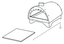
1 - Insert refractory brick into the oven
